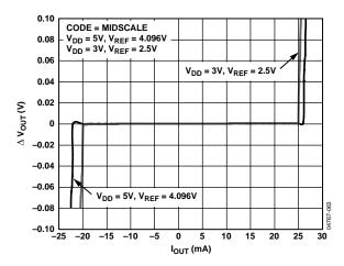
Figure 36. Typical Current Limiting Plot
