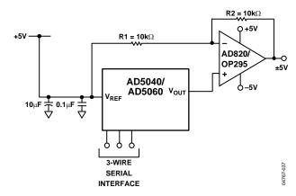
Figure 51. Bipolar Operation with the AD5040/AD5060
