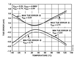
Figure 17. Typical TUE Error vs. Temperature<sup>1</sup>
