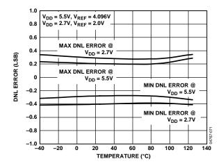
Figure 16. Typical DNL Error vs. Temperature<sup>1</sup>
