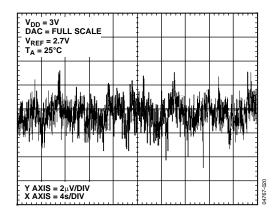
Figure 25. 0.1 Hz to 10 Hz Noise Plot
