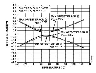
Figure 13. Typical Offset Error vs. Temperature<sup>1</sup>
