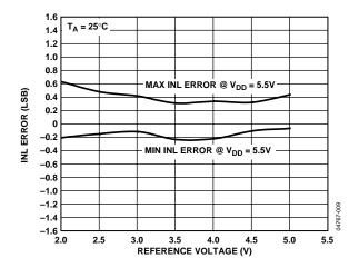
Figure 10. INL vs. Reference Input Voltage<sup>1</sup>
