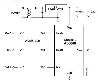
Figure 52. AD5040/AD5060 with a Galvanically Isolated Interface
