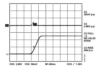
Figure 34. Glitch upon Exiting Hardware Power-Down to Zero Scale
