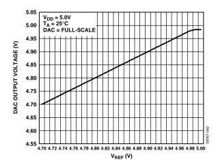
Figure 27. Output Voltage vs. Reference Voltage
