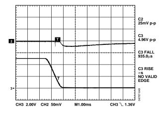
Figure 33. Glitch upon Entering Hardware Power-Down to Three-State
