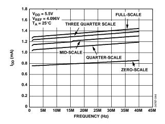
Figure 19. Typical Supply Current vs. Frequency @ 5.5 V1
