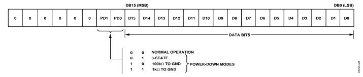
Figure 41. AD5060 Input Register Content
