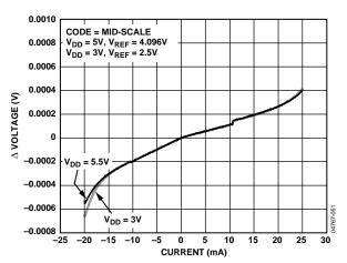
Figure 35. Typical Output Load Regulation
