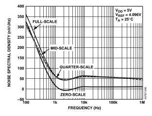
Figure 30. Noise Spectral Density
