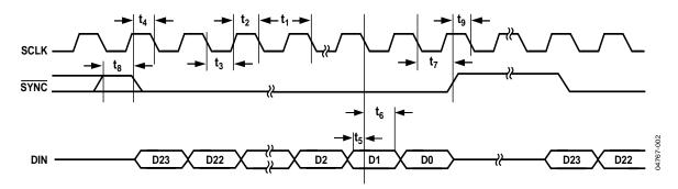
Figure 2. AD5060 Timing Diagram
