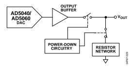
Figure 44. Output Stage During Power-Down
