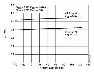
Figure 18. Typical Supply Current vs. Temperature<sup>1</sup>
