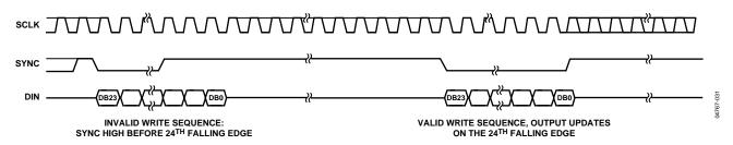
Figure 43. AD5060 SYNC Interrupt Facility
