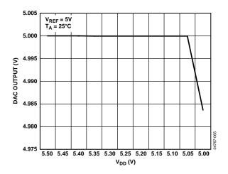
Figure 28. Typical Output vs. Supply Voltage
