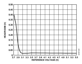
Figure 26. V<sub>DD</sub> Headroom vs. Reference Voltage
