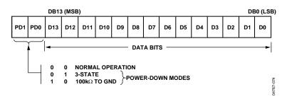
Figure 42. AD5040 Input Register Content
