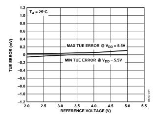
Figure 12. TUE vs. Reference Input Voltage<sup>1</sup>
