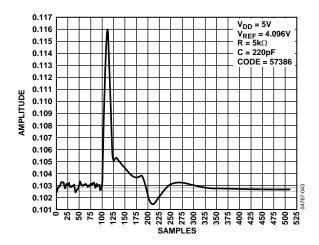
Figure 24. AD5060 Digital-to-Analog Glitch Energy
