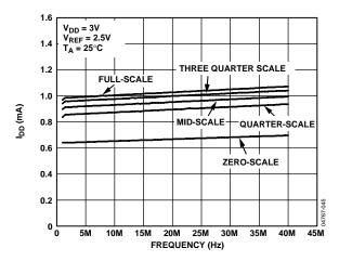
Figure 20. Typical Supply Current vs. Frequency @ 3 V<sup>1</sup>
