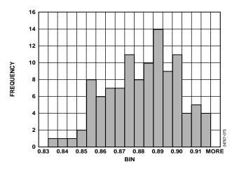
Figure 38.  $I_{DD}$  Histogram  $V_{DD} = 3.0 \text{ V}$
