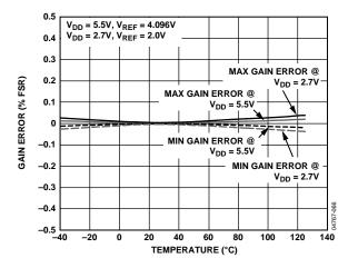
Figure 14. Typical Gain Error vs. Temperature<sup>1</sup>
