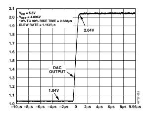
Figure 37. Typical Output Slew Rate
