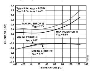
Figure 15. Typical INL Error vs. Temperature<sup>1</sup>
