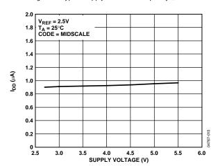
Figure 21. Typical Supply Current vs. Supply Voltage<sup>1</sup>
