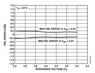
Figure 11. DNL vs. Reference Input Voltage<sup>1</sup>
